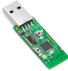
Figura 14: CC2531 Módulo USB-Zigbee Dongle
